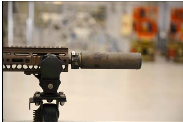
Figure 2: A typical sound suppresser for a small caliber weapon.
