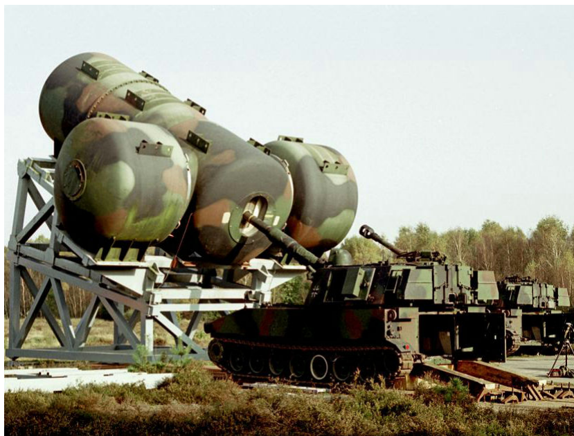
Figure 4: A silencer developed by the German Army to suppress the noise from 155 mm howitzer cannon.
